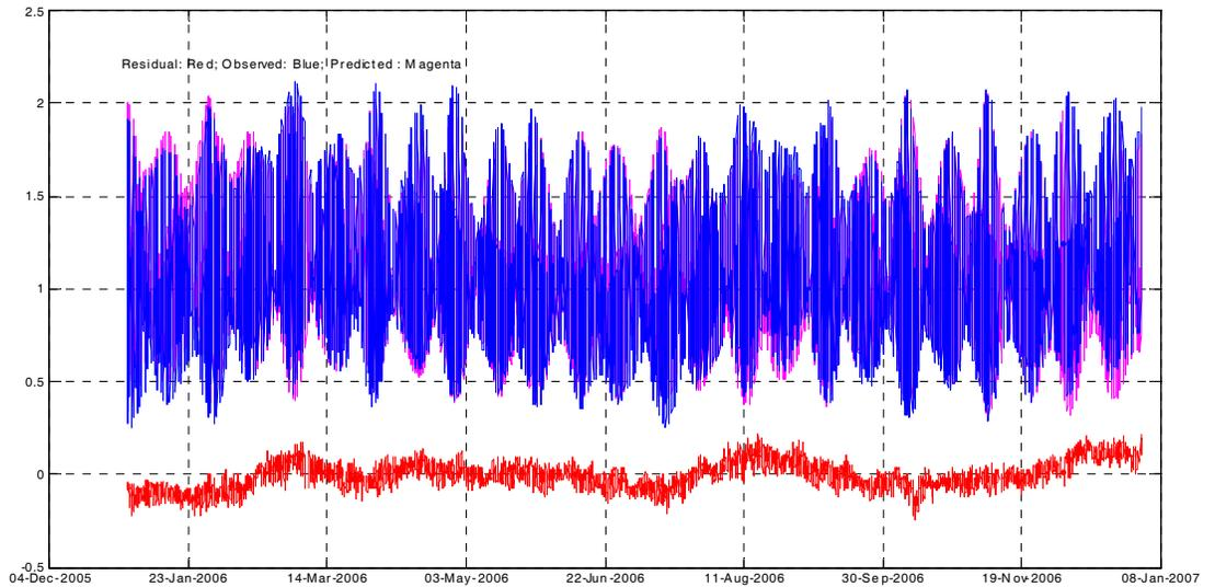
Figure 5: Graphs of observed (blue), predicted (magenta) and residual (red) using 2003 hourly sea level data for Pointe Larue station by T\_TIDE.
