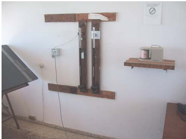
Figure 7. Airport mercury column barometers with WMO reported elevation at column base as 4.58m above sea level.
