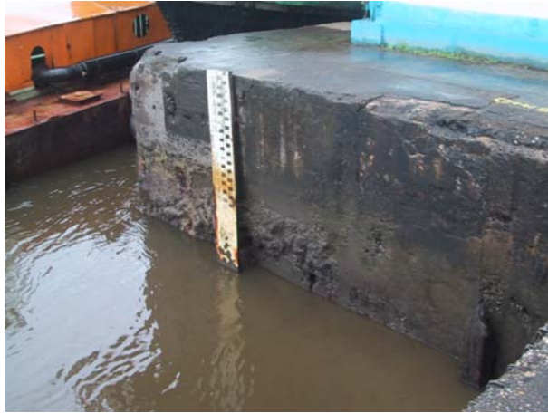
Figure 11. Kribi Port tide staff with the benchmark in yellow paint (top right)
