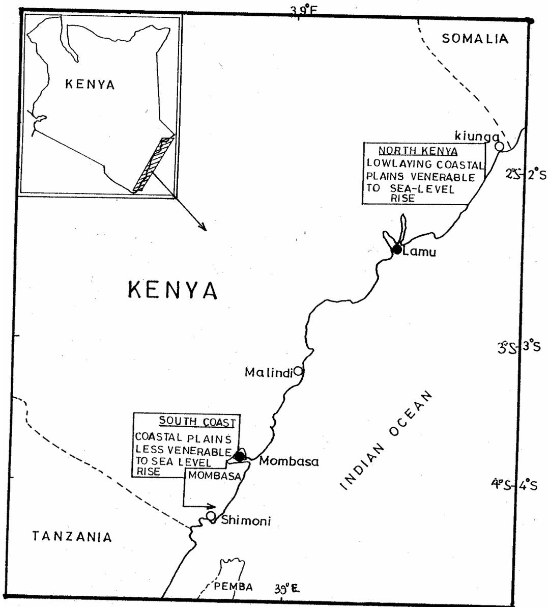
Fig:1. Map of Kenya Coastline showing location of installed tide gauge stations(●)and planned stations(O)
