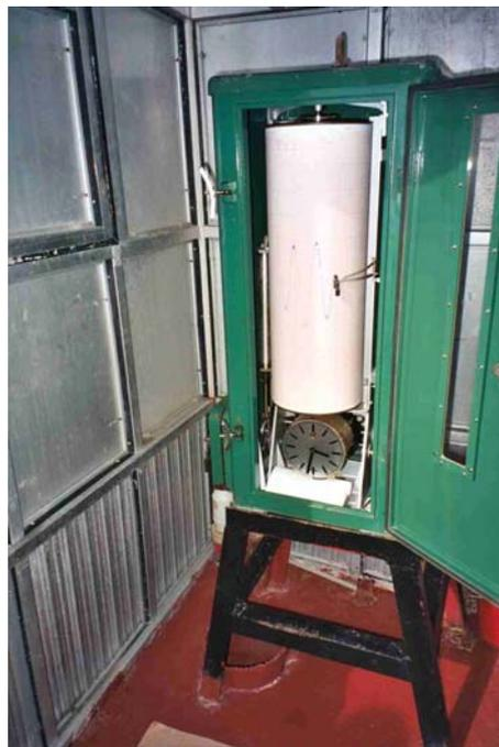
Figure 8. Float gauge manufactured by the Ott company.
