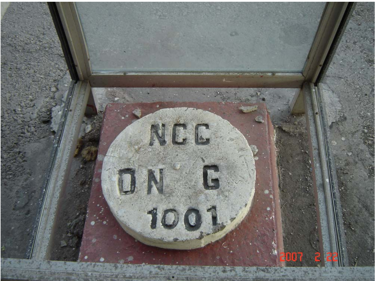
Fig. 7 Shahid Rajae Bench mark of the leveling network
