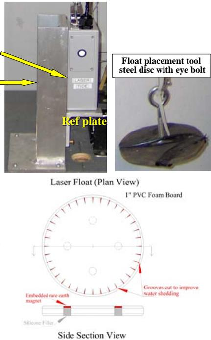
Figure 6: The Laser-Float Sensor
