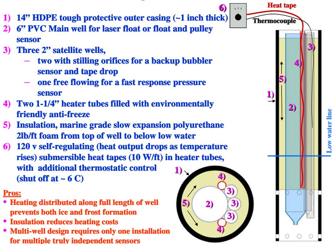
Figure 5: The Insulated, Heated Multi-well Stilling Well
