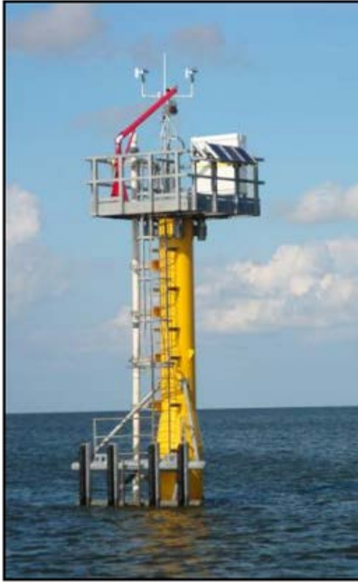
Figure 13. One of the US NOAA Sentinel Tide Stations in the Gulf of Mexico.
