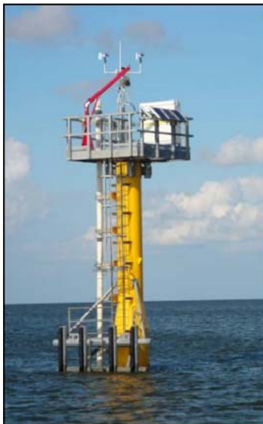
Figure 12. One of the US NOAA Sentinel Tide Stations in the Gulf of Mexico.
