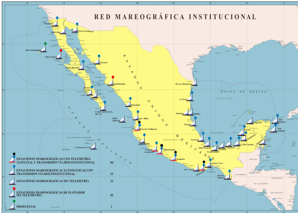
Figure 2. Distribution of Mexican Navy sea level stations. (black) sites with satellite telemetry, (blue) sites with internal Navy network communication, (no color) sites without telemetry, (red) sites with float sensor without telemetry, and (green) planned sites.
