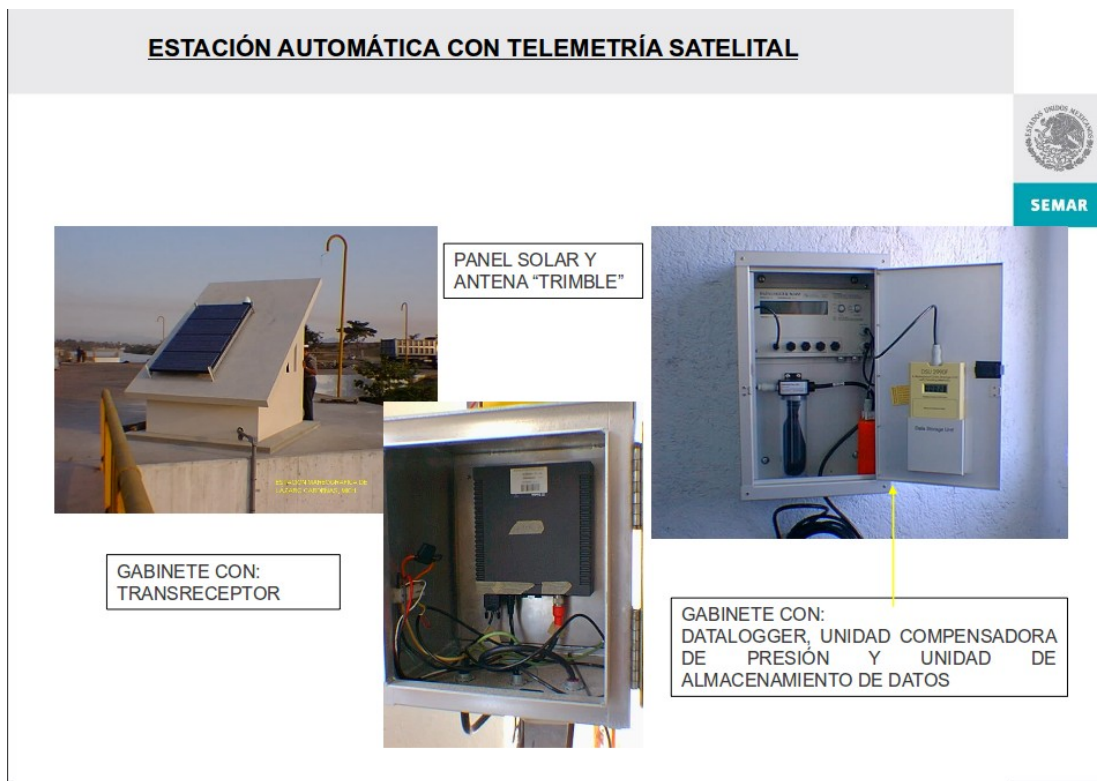
Figure 3. Example of the Mexican navy station showing solar panel and trimble antenna, transmitter and datalogger including atmospheric pressure compensator.
