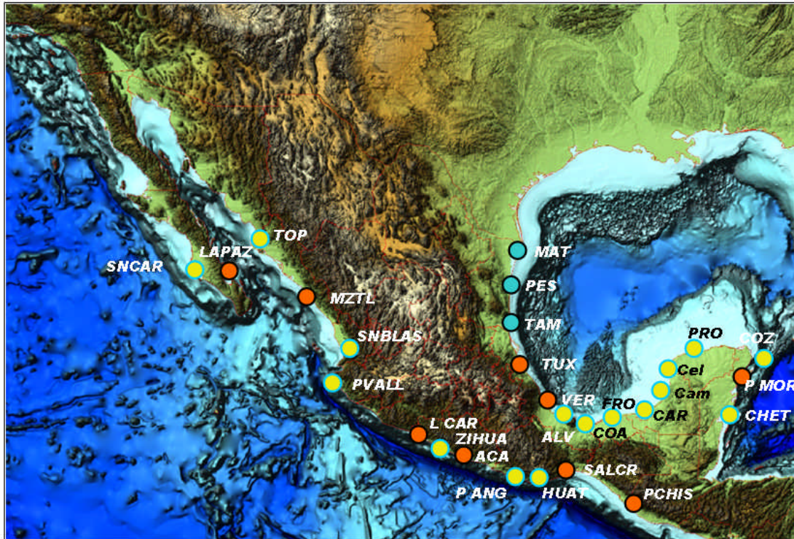
Figure 1. UNAM Sea level Network. Red dots are sites rehabilitated and working, yellow dots are sites planned to be rehabilitated in 2009-2010. With blue are the sites operated by CICATA.
