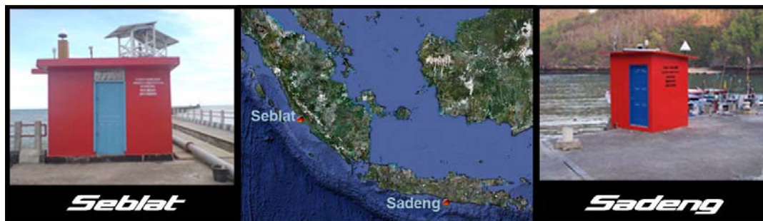
Figure 4. The tidal huts with GPS antenna on top located in Seblat (Sumatra) and Sadeng (Java).
